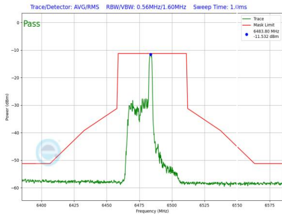
Plot 7-1452. LPI In-Band Emission Plot SDM Diversity Antenna 2a (40MHz 802.11ax RU26 (UNII Band 6) – Ch. 107)
