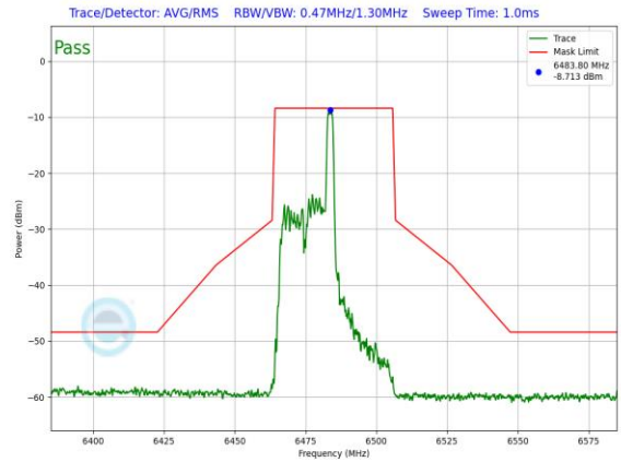
Plot 7-1174. LPI In-Band Emission Plot Antenna 4a (40MHz 802.11ax RU26 (UNII Band 6) – Ch. 107)
