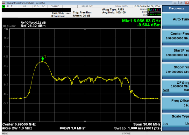
Plot 7-706. LPI Power Spectral Density Plot SDM Primary Antenna 4a (20MHz 802.11ax RU26 (UNII Band 8) – Ch. 209)
