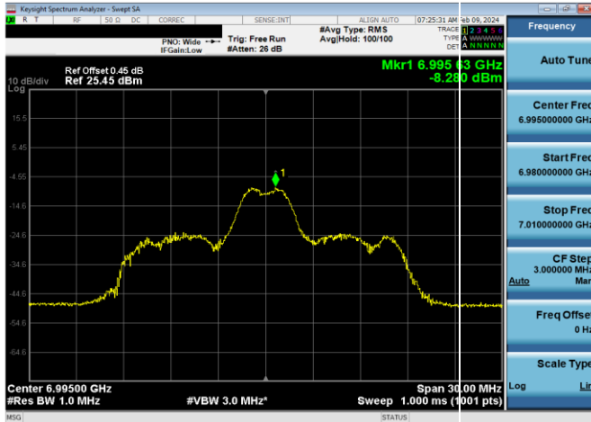
Plot 7-594. LPI Power Spectral Density Plot Antenna 2a (20MHz 802.11ax RU26 (UNII Band 8) – Ch. 209)
