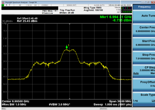
Plot 7-466. LPI Power Spectral Density Plot Antenna WF5B (20MHz 802.11ax RU26 (UNII Band 8) – Ch. 209)
