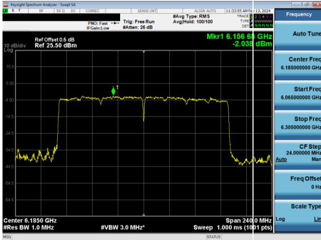
Plot 7-383. SP Power Spectral Density Plot CDD Diversity Antenna 4a (160MHz 802.11ax RU996x2 (UNII Band 5) – Ch. 47)
