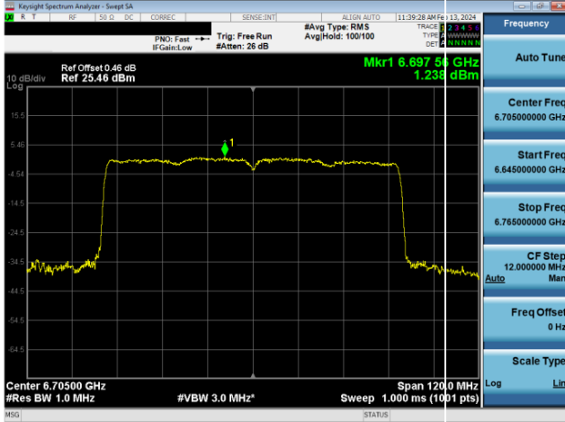
Plot 7-407. SP Power Spectral Density Plot CDD Diversity Antenna 4a (80MHz 802.11ax RU996 (UNII Band 7) - Ch. 151)
