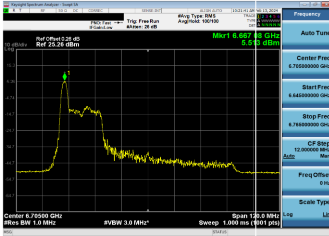
Plot 7-249. SP Power Spectral Density Plot Antenna 4a (80MHz 802.11ax RU26 (UNII Band 7) – Ch. 151)
