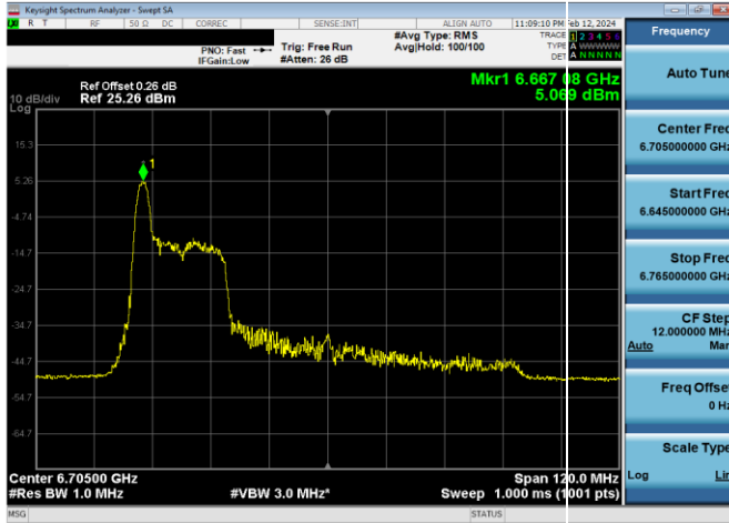
Plot 7-217. SP Power Spectral Density Plot Antenna WF5B (80MHz 802.11ax RU26 (UNII Band 7) – Ch. 151)
