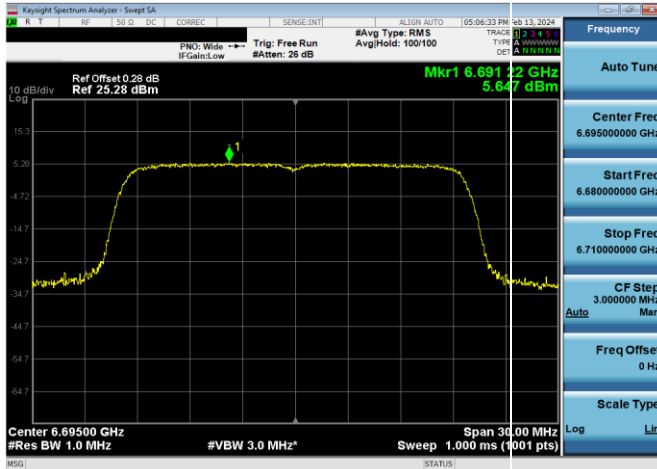
Plot 7-276. SP Power Spectral Density Plot Antenna 2a (20MHz 802.11ax RU242 (UNII Band 7) – Ch. 149)
