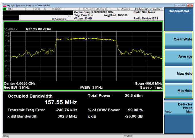
Plot 7-176. 26dB & 99% Bandwidth Plot Antenna 2a (160MHz 802.11ax RU996x2 (UNII Band 7) – Ch. 143)
