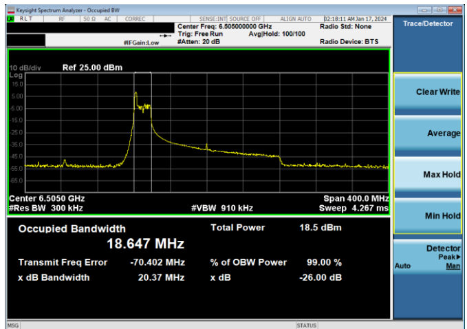
Plot 7-157. 26dB & 99% Bandwidth Plot Antenna 2a (160MHz 802.11ax RU26 (UNII Band 6) – Ch. 111)
