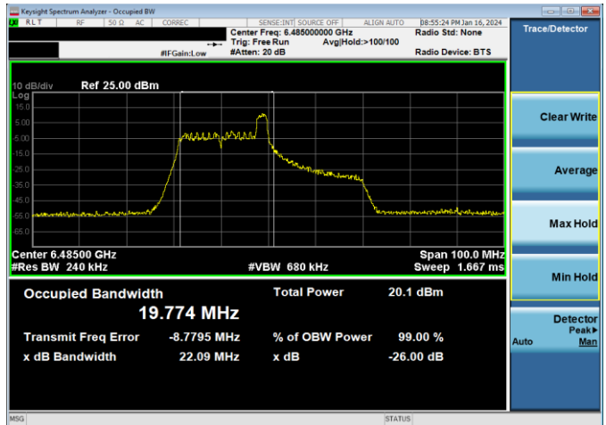
Plot 7-86. 26dB & 99% Bandwidth Plot Antenna 4a (40MHz 802.11ax RU26 (UNII Band 6) – Ch. 107)
