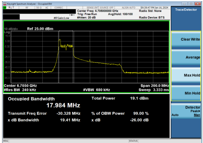
Plot 7-105. 26dB & 99% Bandwidth Plot Antenna 4a (80MHz 802.11ax RU26 (UNII Band 7) – Ch. 151)
