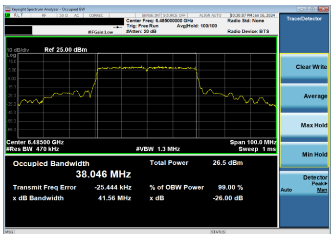
Plot 7-88. 26dB & 99% Bandwidth Plot Antenna 4a (40MHz 802.11ax RU484 (UNII Band 6) – Ch. 107)
