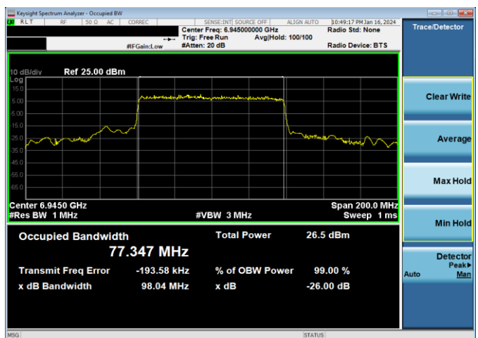
Plot 7-124. 26dB & 99% Bandwidth Plot Antenna 4a (80MHz 802.11ax RU996 (UNII Band 8) – Ch. 199)
