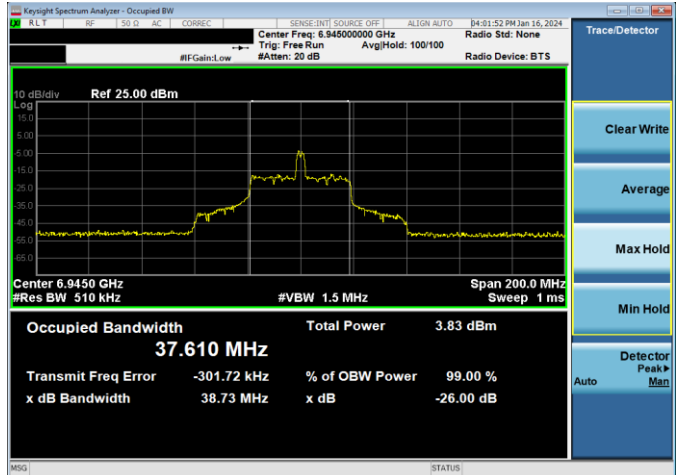
Plot 7-58. 26dB & 99% Bandwidth Plot Antenna WF5B (80MHz 802.11ax RU26 (UNII Band 8) – Ch. 199)
