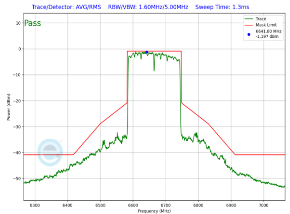
Plot 7-936. SP In-Band Emission Plot Antenna 2a (160MHz 802.11ax (UNII Band 7) – Ch. 143, MCS11)
