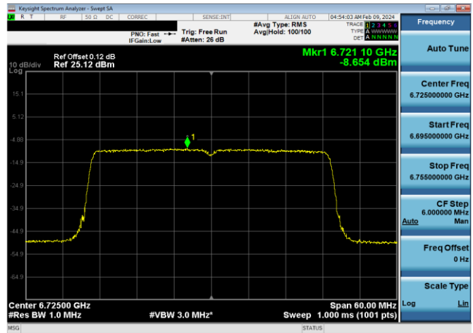
Plot 7-604. Power Spectral Density Plot SDM Diversity Antenna 2a LPI (40MHz 802.11ax (UNII Band 7) – Ch. 155, MCS2)
