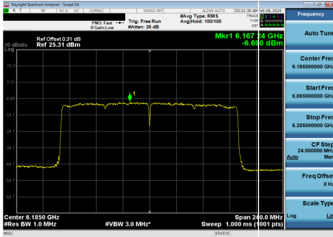
Plot 7-489. Power Spectral Density Plot SDM Primary Antenna WF5B LPI (160MHz 802.11ax (UNII Band 5) – Ch. 47, MCS4)
