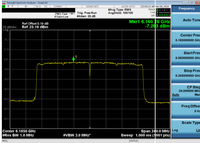
Plot 7-457. Power Spectral Density Plot SDM Primary Antenna WF5B LPI (160MHz 802.11ax (UNII Band 5) – Ch. 47, MCS2)
