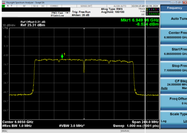
Plot 7-513. Power Spectral Density Plot SDM Primary Antenna WF5B LPI (160MHz 802.11ax (UNII Band 8) – Ch. 207, MCS4)
