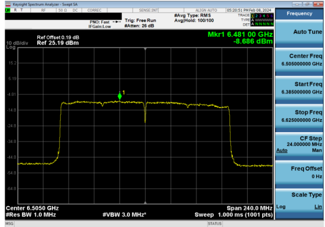
Plot 7-466. Power Spectral Density Plot SDM Primary Antenna 4a LPI (160MHz 802.11ax (UNII Band 6) – Ch. 111, MCS2)
