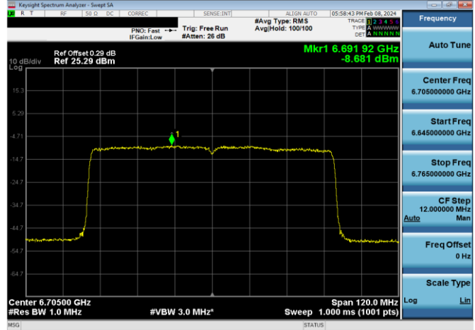
Plot 7-504. Power Spectral Density Plot SDM Primary Antenna 4a LPI (80MHz 802.11ax (UNII Band 7) – Ch. 151, MCS4)
