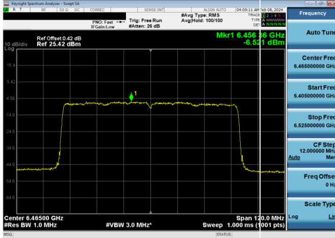
Plot 7-527. Power Spectral Density Plot SDM Primary Antenna WF5B LPI (80MHz 802.11ax (UNII Band 6) – Ch. 103, MCS11)
