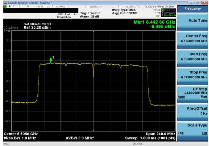
Plot 7-390. Power Spectral Density Plot Antenna 2a LPI (160MHz 802.11ax (UNII Band 6) – Ch. 111, MCS4)
