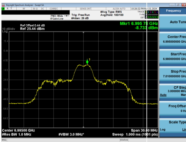
Plot 7-835. LPI Power Spectral Density Plot SDM Diversity Antenna WF8 (20MHz 802.11ax RU26 (UNII Band 8) – Ch. 209)
