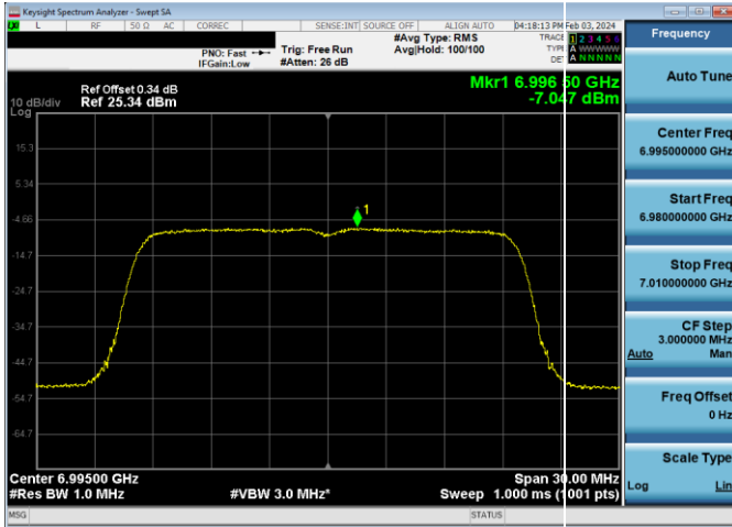
Plot 7-711. LPI Power Spectral Density Plot SDM Primary Antenna WF5B (20MHz 802.11ax RU242 (UNII Band 8) – Ch. 209)
