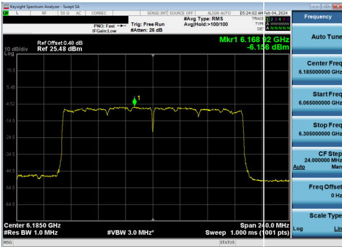
Plot 7-640. LPI Power Spectral Density Plot SDM Primary Antenna WF5B (160MHz 802.11ax RU996x2 (UNII Band 5) – Ch. 47)
