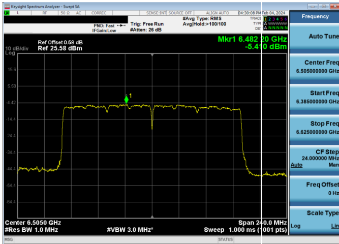
Plot 7-576. LPI Power Spectral Density Plot Antenna WF7 (160MHz 802.11ax RU996x2 (UNII Band 6) – Ch. 111)
