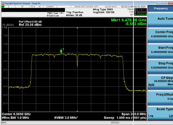
Plot 7-512. LPI Power Spectral Density Plot Antenna WF8 (160MHz 802.11ax RU996x2 (UNII Band 6) – Ch. 111)
