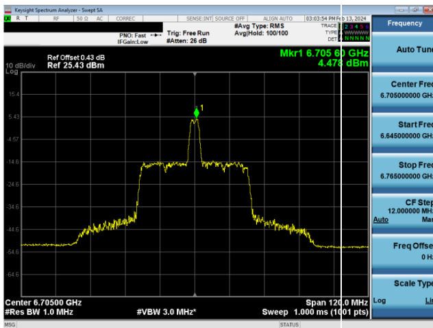
Plot 7-403. SP Power Spectral Density Plot CDD Diversity Antenna WF8 (80MHz 802.11ax RU26 (UNII Band 7) – Ch. 151)
