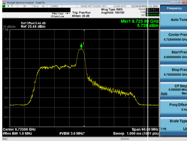
Plot 7-395. SP Power Spectral Density Plot CDD Diversity Antenna WF6 (40MHz 802.11ax RU26 (UNII Band 7) - Ch. 155)
