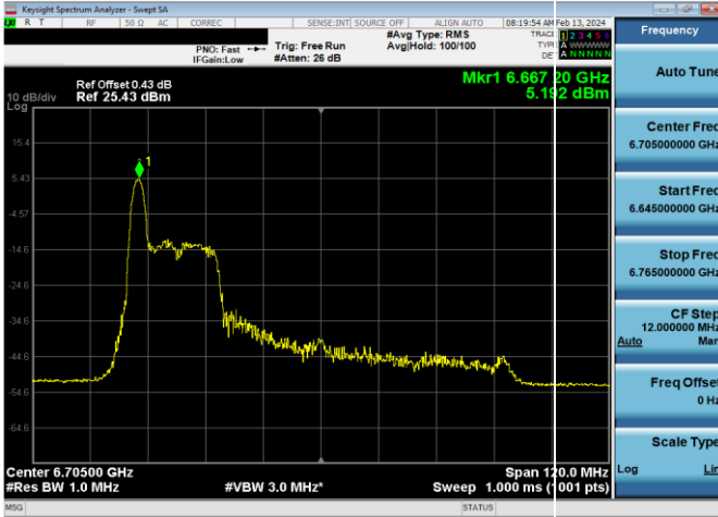
Plot 7-337. SP Power Spectral Density Plot CDD Primary Antenna WF5B (80MHz 802.11ax RU26 (UNII Band 7) – Ch. 151)
