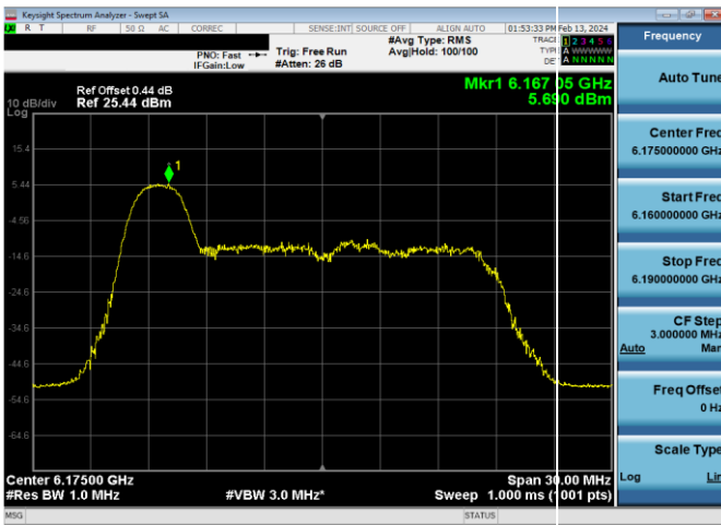
Plot 7-290. SP Power Spectral Density Plot CDD Primary Antenna WF8 (20MHz 802.11ax RU26 (UNII Band 5) - Ch. 45)
