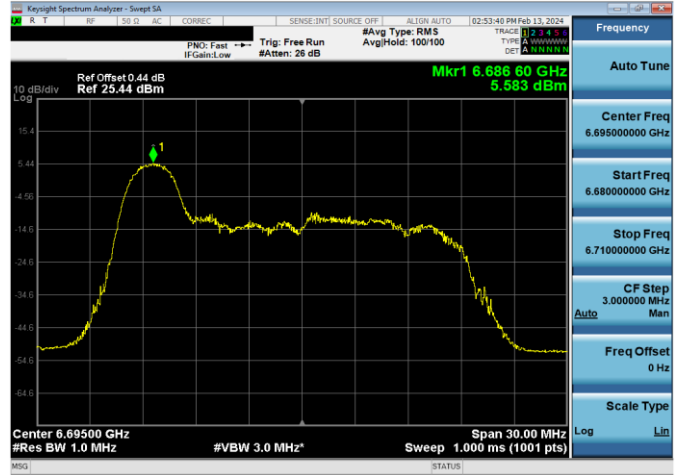
Plot 7-322. SP Power Spectral Density Plot CDD Primary Antenna WF8 (20MHz 802.11ax RU26 (UNII Band 7) – Ch. 149)
