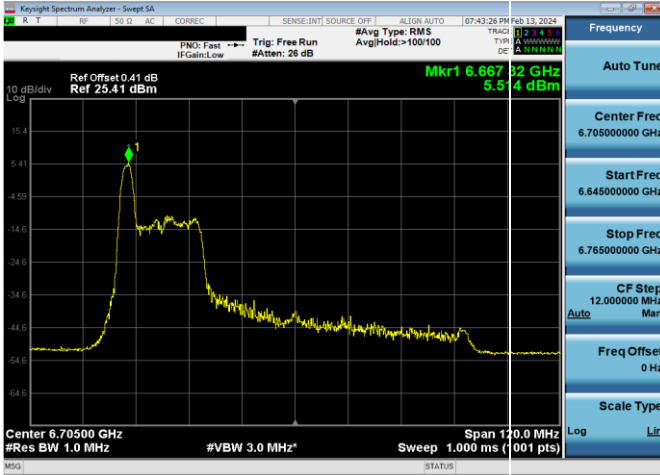
Plot 7-281. SP Power Spectral Density Plot Antenna WF7 (80MHz 802.11ax RU26 (UNII Band 7) – Ch. 151)
