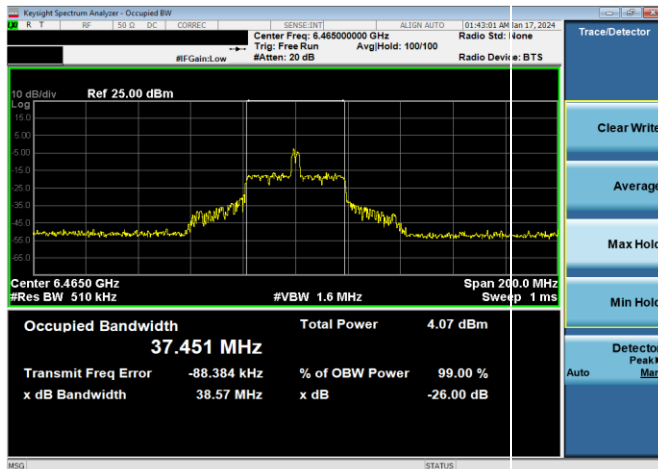
Plot 7-154. 26dB & 99% Bandwidth Plot Antenna WF7 (80MHz 802.11ax RU26 (UNII Band 6) – Ch. 103)
