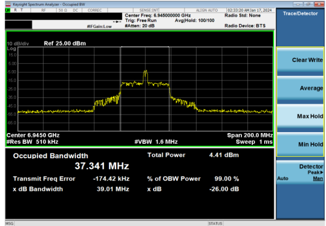
Plot 7-186. 26dB & 99% Bandwidth Plot Antenna WF7 (80MHz 802.11ax RU26 (UNII Band 8) – Ch. 199)
