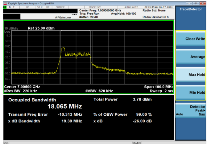
Plot 7-181. 26dB & 99% Bandwidth Plot Antenna WF7 (40MHz 802.11ax RU26 (UNII Band 8) – Ch. 211)
