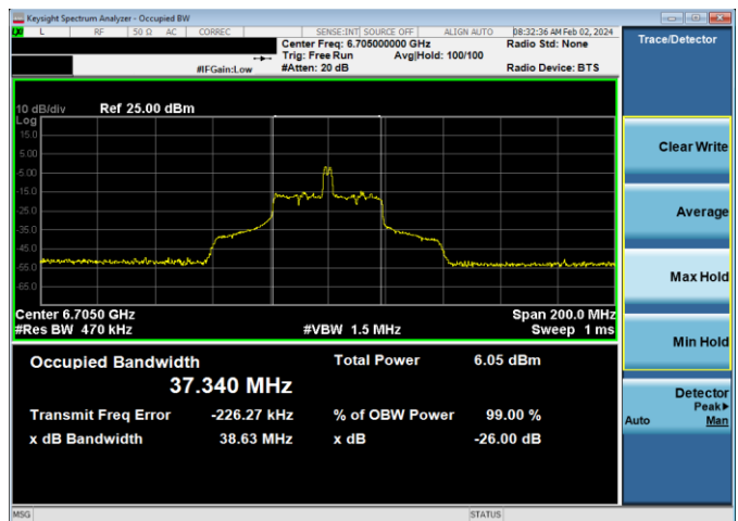
Plot 7-106. 26dB & 99% Bandwidth Plot Antenna WF8 (80MHz 802.11ax RU26 (UNII Band 7) – Ch. 151)
