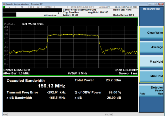
Plot 7-112. 26dB & 99% Bandwidth Plot Antenna WF8 (160MHz 802.11ax RU484 (UNII Band 7) – Ch. 143)
