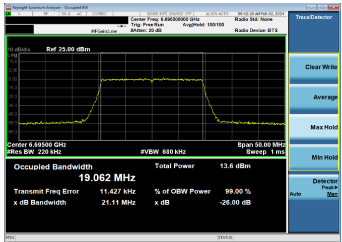
Plot 7-100. 26dB & 99% Bandwidth Plot Antenna WF8 (20MHz 802.11ax RU242 (UNII Band 7) – Ch. 149)
