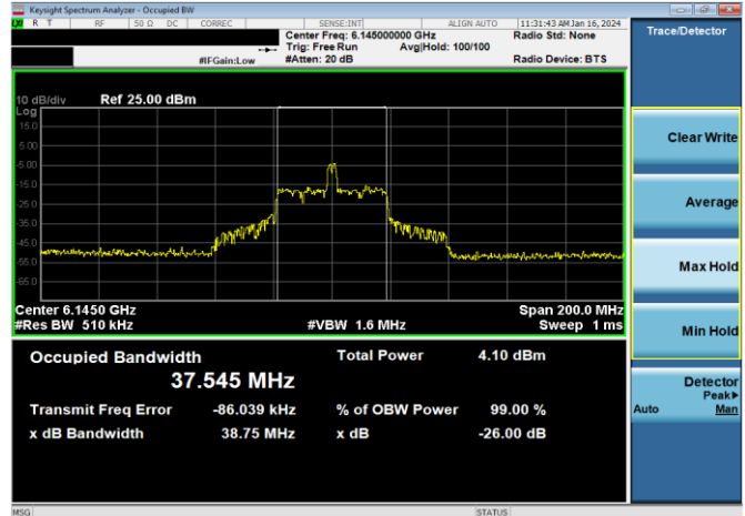
Plot 7-10. 26dB & 99% Bandwidth Plot Antenna WF5B (80MHz 802.11ax RU26 (UNII Band 5) – Ch. 39)
