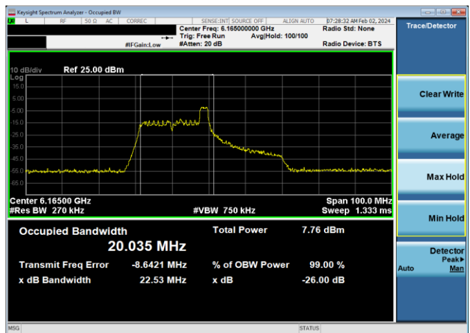
Plot 7-70. 26dB & 99% Bandwidth Plot Antenna WF8 (40MHz 802.11ax RU26 (UNII Band 5) – Ch. 43)
