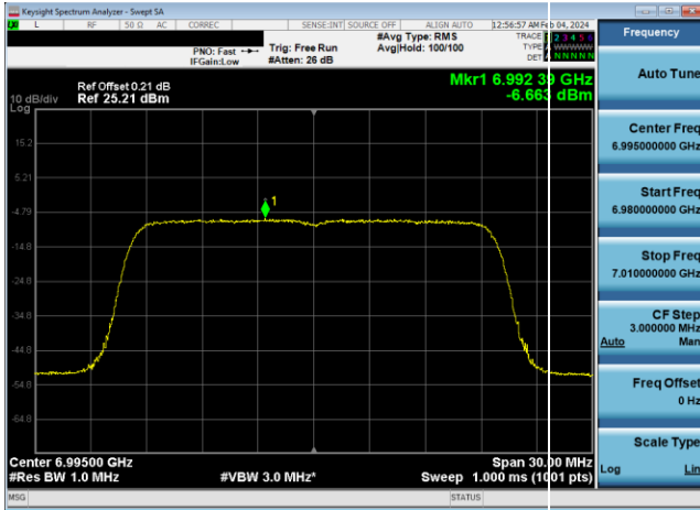
Plot 7-652. Power Spectral Density Plot SDM Diversity Antenna WF8 LPI (20MHz 802.11ax (UNII Band 8) – Ch. 209, MCS4)
