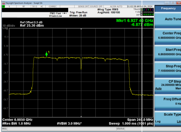
Plot 7-658. Power Spectral Density Plot SDM Diversity Antenna WF8 LPI (160MHz 802.11ax (UNII Band 8) – Ch. 207, MCS4)
