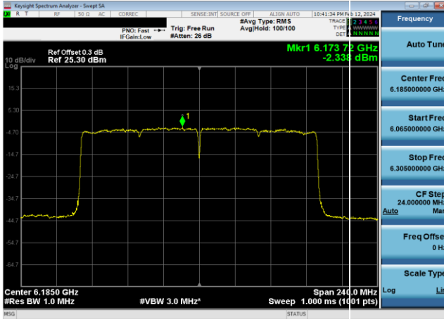
Plot 7-570. Power Spectral Density Plot CDD Primary Antenna WF5B Standard Power (160MHz 802.11ax (UNII Band 5) – Ch. 47, MCS4)
