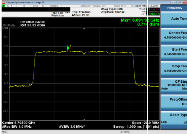
Plot 7-592. Power Spectral Density Plot CDD Primary Antenna WF5B Standard Power (80MHz 802.11ax (UNII Band 7) – Ch. 151, MCS11)
