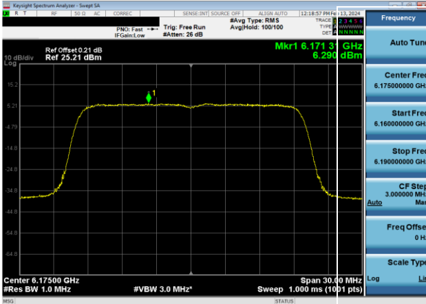
Plot 7-565. Power Spectral Density Plot CDD Primary Antenna WF8 Standard Power (20MHz 802.11ax (UNII Band 5) – Ch. 45, MCS4)
