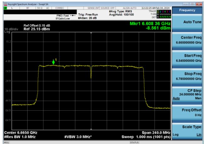
Plot 7-618. Power Spectral Density Plot SDM Diversity Antenna WF8 LPI (160MHz 802.11ax (UNII Band 7) – Ch. 143, MCS2)
