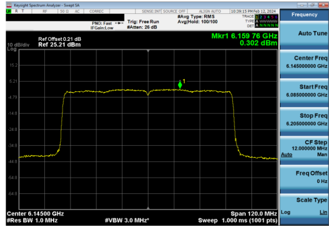
Plot 7-568. Power Spectral Density Plot CDD Primary Antenna WF5B Standard Power (80MHz 802.11ax (UNII Band 5) – Ch. 39, MCS4)
