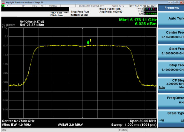
Plot 7-580. Power Spectral Density Plot CDD Primary Antenna WF5B Standard Power (20MHz 802.11ax (UNII Band 5) – Ch. 45, MCS11)
