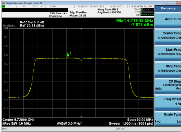
Plot 7-614. Power Spectral Density Plot SDM Diversity Antenna WF8 LPI (40MHz 802.11ax (UNII Band 7) – Ch. 155, MCS2)
