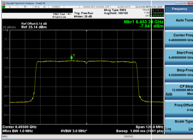
Plot 7-608. Power Spectral Density Plot SDM Diversity Antenna WF8 LPI (80MHz 802.11ax (UNII Band 6) – Ch. 103, MCS2)
