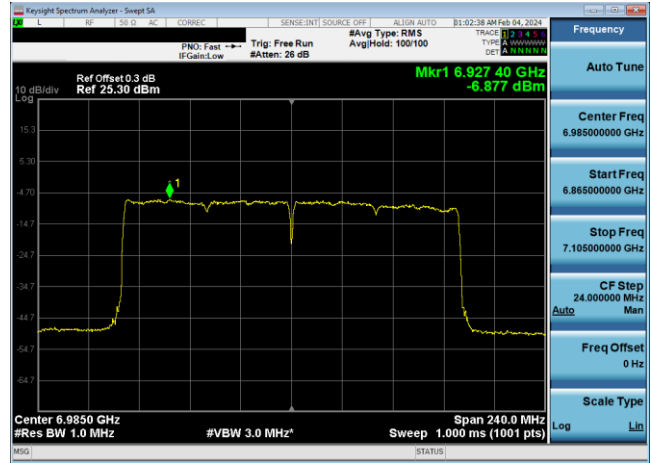
Plot 7-515. Power Spectral Density Plot SDM Primary Antenna WF8 LPI (160MHz 802.11ax (UNII Band 8) – Ch. 207, MCS4)
