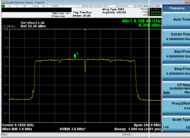
Plot 7-490. Power Spectral Density Plot SDM Primary Antenna WF5B LPI (160MHz 802.11ax (UNII Band 5) – Ch. 47, MCS4)
