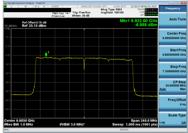
Plot 7-483. Power Spectral Density Plot SDM Primary Antenna WF8 LPI (160MHz 802.11ax (UNII Band 8) – Ch. 207, MCS2)
