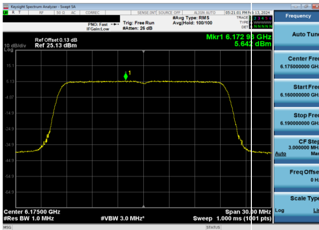
Plot 7-423. Power Spectral Density Plot Antenna WF7 Standard Power (20MHz 802.11ax (UNII Band 5) – Ch. 45, MCS2)
