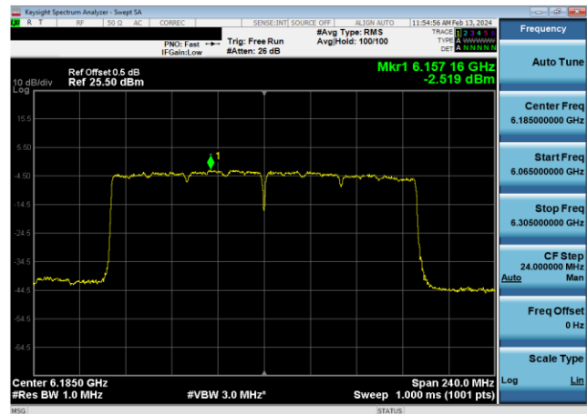
Plot 7-356. Power Spectral Density Plot Antenna WF8 Standard Power (160MHz 802.11ax (UNII Band 5) – Ch. 47, MCS11)
