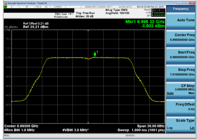
Plot 7-216. Power Spectral Density Plot Antenna WF5B LPI (20MHz 802.11a (UNII Band 8) – Ch. 209, 24Mbps)
