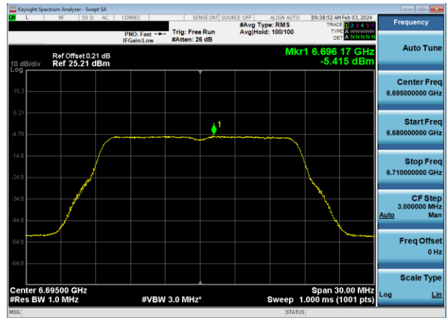
Plot 7-211. Power Spectral Density Plot Antenna WF5B LPI (20MHz 802.11a (UNII Band 7) – Ch. 149, 24Mbps)
