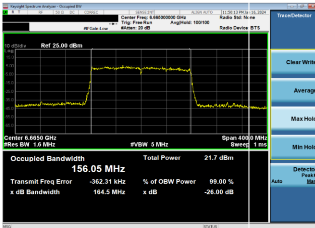
Plot 7-155. 26dB & 99% Bandwidth Plot Antenna WF7 (160MHz 802.11ax (UNII Band 7) – Ch. 143, MCS4)
