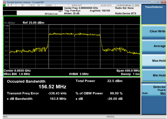
Plot 7-180. 26dB & 99% Bandwidth Plot Antenna WF7 (160MHz 802.11ax (UNII Band 8) – Ch. 207, MCS11)
