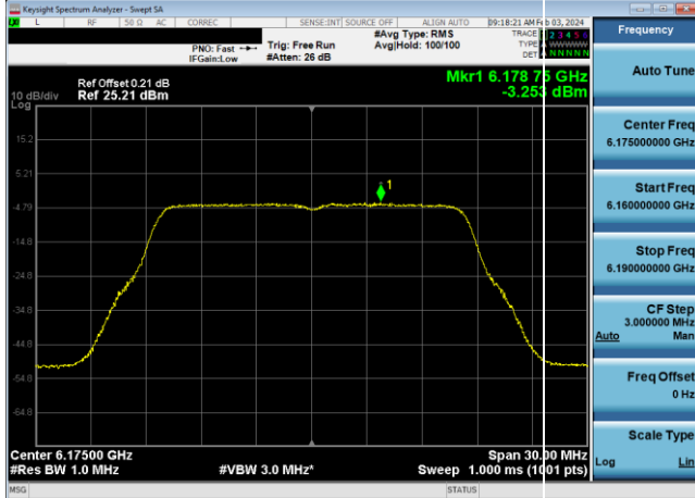
Plot 7-201. Power Spectral Density Plot Antenna WF5B LPI (20MHz 802.11a (UNII Band 5) – Ch. 45, 24Mbps)
