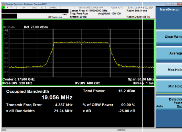
Plot 7-102. 26dB & 99% Bandwidth Plot Antenna WF8 (20MHz 802.11ax (UNII Band 5) – Ch. 45, MCS11)
