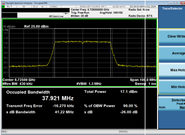
Plot 7-93. 26dB & 99% Bandwidth Plot Antenna WF8 (40MHz 802.11ax (UNII Band 7) – Ch. 155, MCS4)
