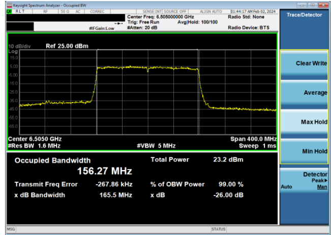
Plot 7-70. 26dB & 99% Bandwidth Plot Antenna WF8 (160MHz 802.11ax (UNII Band 6) – Ch. 111, MCS2)
