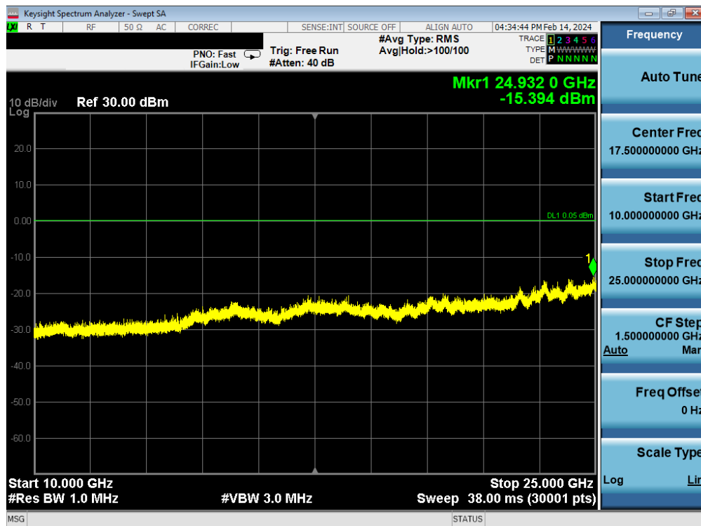
Plot 7-84. Conducted Spurious Plot Antenna WF9 (Bluetooth, GFSK, ePA – Ch. 78)
