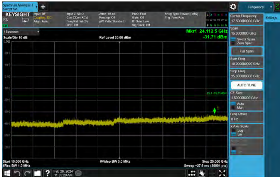
Plot 7-86. Conducted Simultaneous Tx Spurious Plot Antenna WF8 (Bluetooth + UNII)
