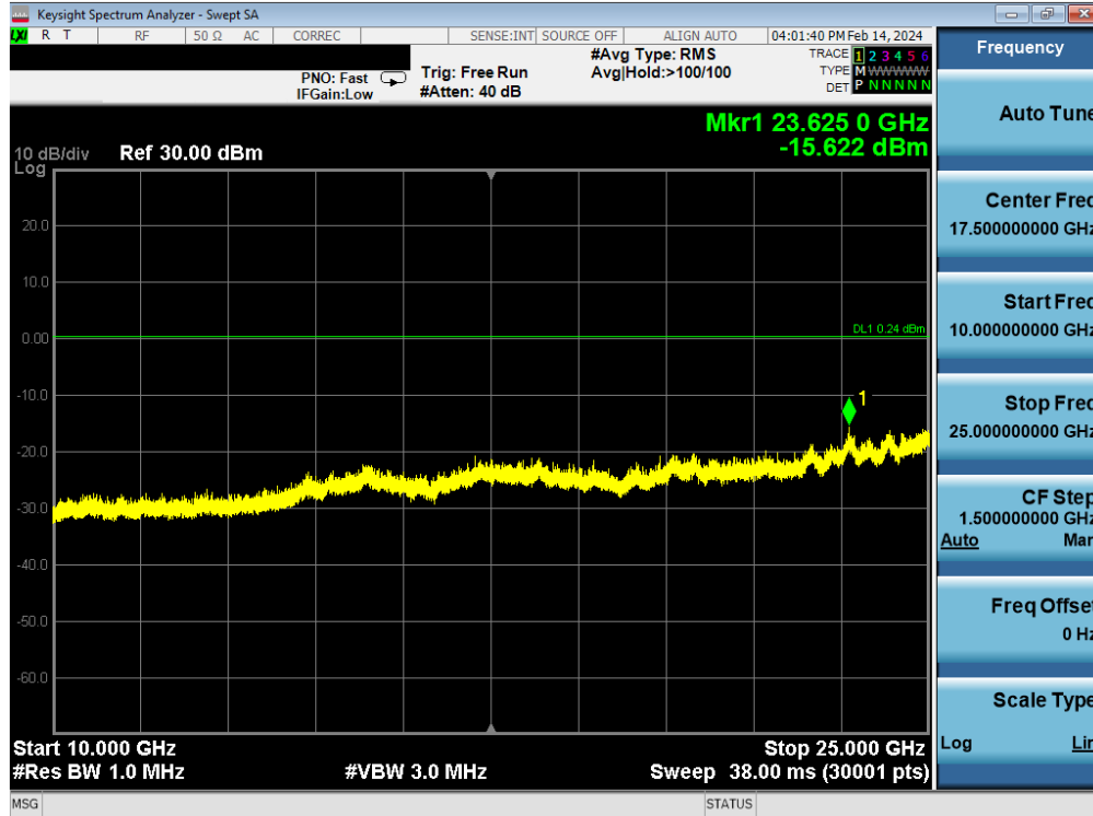
Plot 7-72. Conducted Spurious Plot Antenna WF8 (Bluetooth, GFSK, ePA – Ch. 78)
