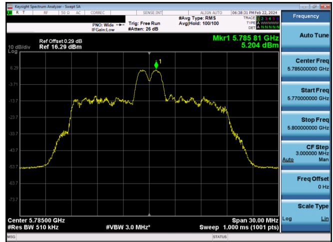
Plot 7-615. PSD CDD Diversity Antenna WF7 (20MHz BW 11ax Index 4 – RU26 – Ch.157)
