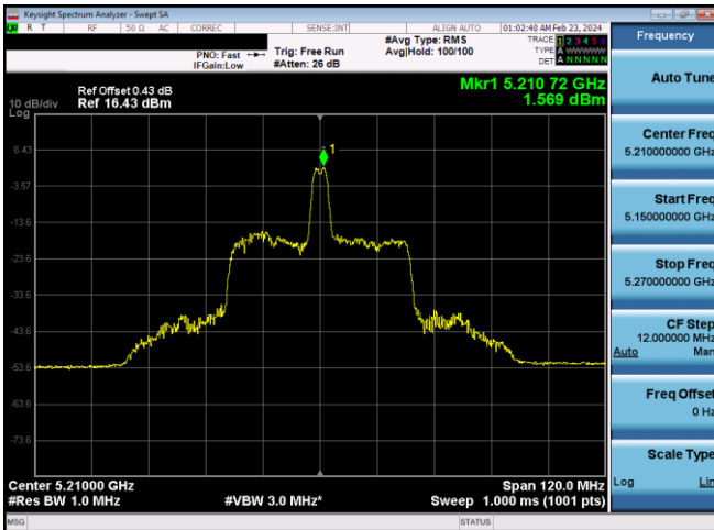
Plot 7-513. ISED PSD SDM Primary Antenna WF8 (80MHz BW 11ax Index 18 - RU26 - Ch.42)
