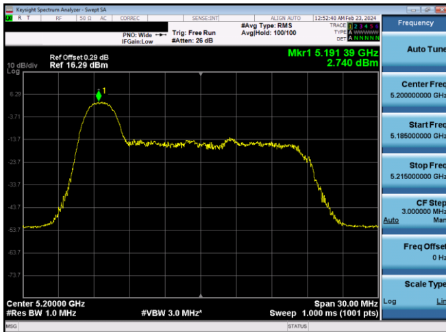
Plot 7-495. ISED PSD SDM Primary Antenna WF8 (20MHz BW 11ax Index 0 - RU26 - Ch.40)
