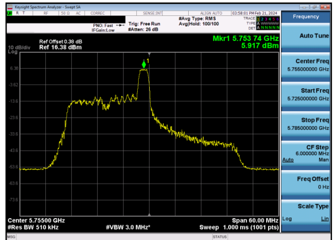
Plot 7-480. PSD CDD Primary Antenna WF5B (40MHz BW 11ax Index 8 - RU26 - Ch.151)
