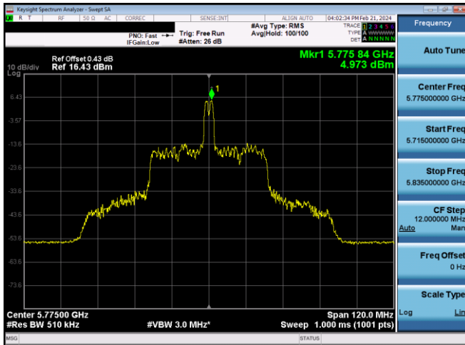
Plot 7-488. PSD CDD Primary Antenna WF5B (80MHz BW 11ax Index 18 – RU26 – Ch.155)
