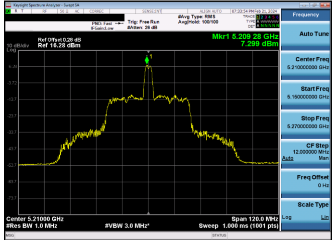
Plot 7-249. PSD Antenna WF8 (80MHz BW 11ax Index 18 - RU26 - Ch.42)
