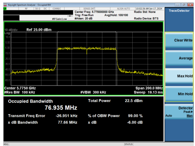
Plot 7-168. 6dB BW & 99% OBW Antenna WF7 (80MHz BW 11ax – RU996 – Ch.155)
