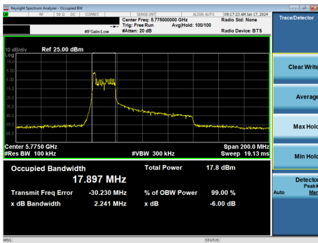
Plot 7-165. 6dB BW & 99% OBW Antenna WF7 (80MHz BW 11ax Index 0 – RU26 – Ch.155)
