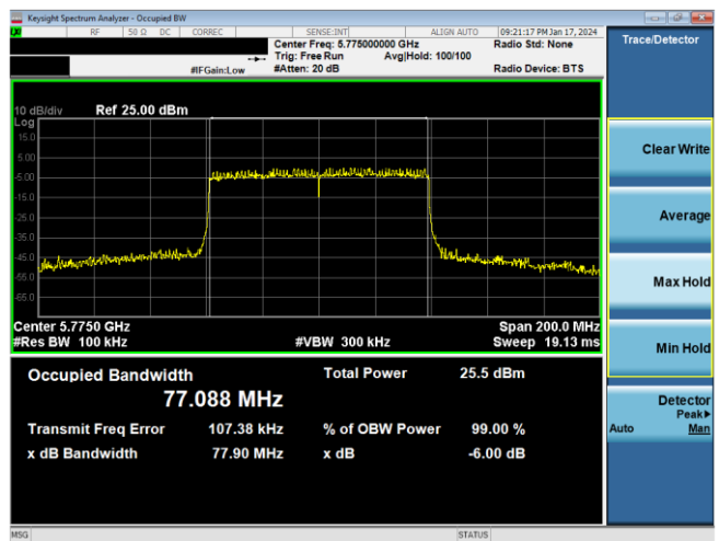
Plot 7-156. 6dB BW & 99% OBW Antenna WF8 (80MHz BW 11ax – RU996 – Ch.155)
