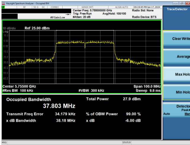
Plot 7-152. 6dB BW & 99% OBW Antenna WF8 (40MHz BW 11ax – RU484 – Ch.151)
