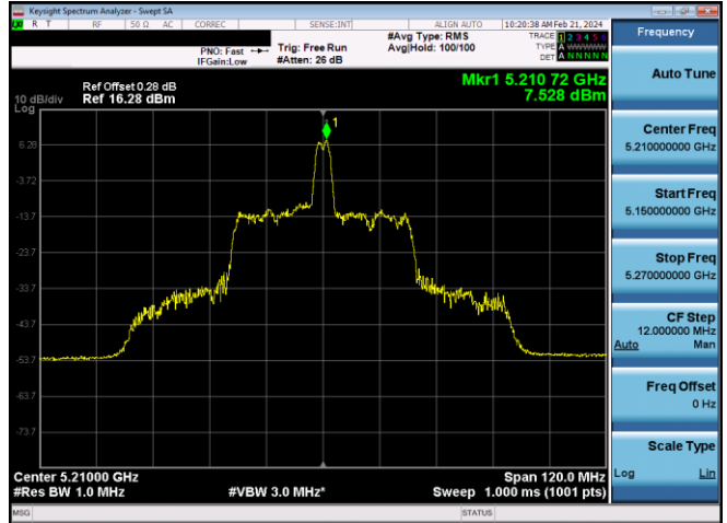
Plot 7-178. PSD Antenna WF5B (80MHz BW 11ax Index 18 - RU26 - Ch.42)
