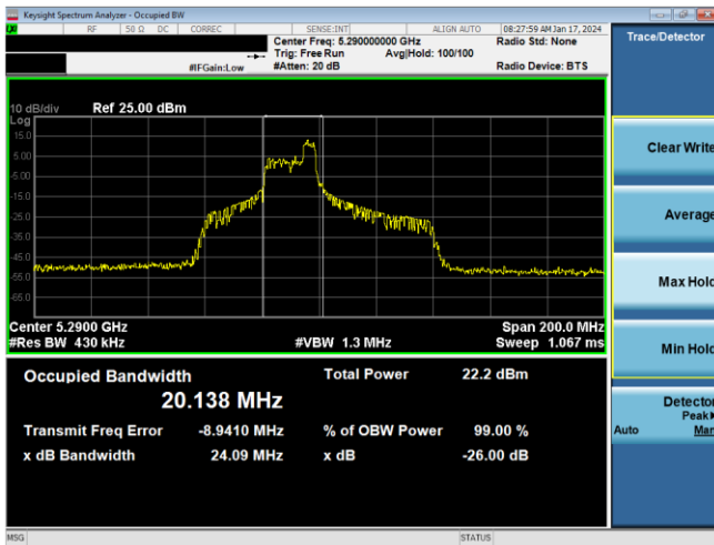
Plot 7-114. 26dB BW & 99% OBW Antenna WF7 (80MHz BW 11ax Index 44 – RU52 – Ch.58)
