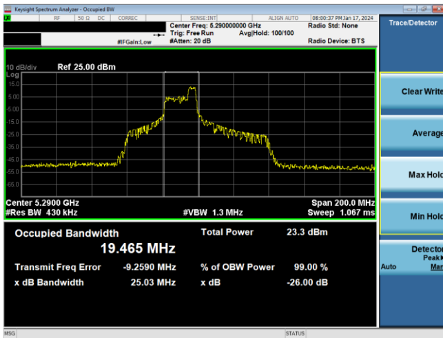
Plot 7-70. 26dB BW & 99% OBW Antenna WF8 (80MHz BW 11ax Index 44 – RU52 – Ch.58)
