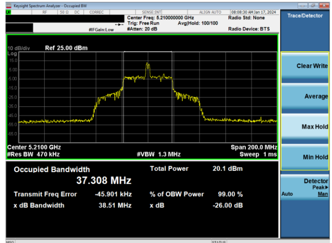
Plot 7-98. 26dB BW & 99% OBW Antenna WF7 (80MHz BW 11ax Index 18 – RU26 – Ch.42)
