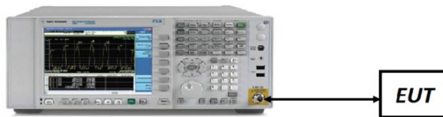
Figure 7-2. Test Instrument & Measurement Setup
