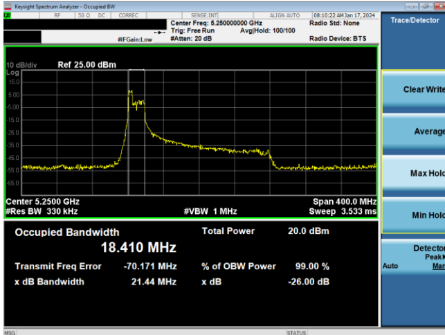
Plot 7-101. 26dB BW & 99% OBW Antenna WF7 (160MHz BW 11ax Index 37 – RU52 – Ch.50 (L))
