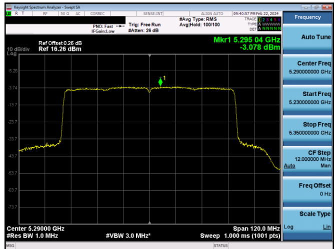
Plot 7-816. PSD CDD DIVERSITY Antenna WF7 (80MHz BW 802.11ax(SU) – Ch. 58, MCS4)
