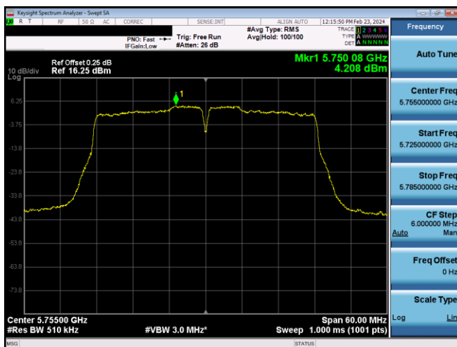
Plot 7-849. PSD CDD DIVERSITY Antenna WF7 (40MHz BW 802.11n – Ch. 151, MCS10)
