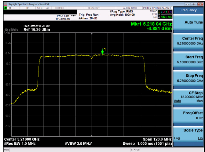
Plot 7-808. PSD CDD DIVERSITY Antenna WF7 (80MHz BW 802.11ax(SU) – Ch. 42, MCS4)
