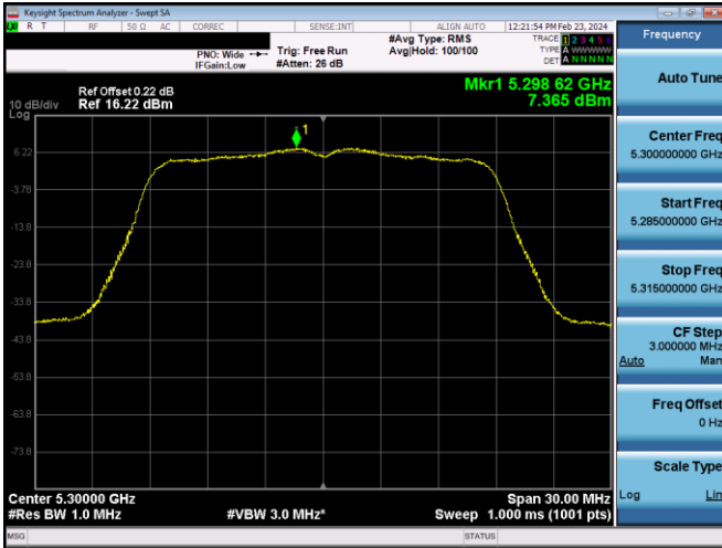
Plot 7-811. PSD CDD DIVERSITY Antenna WF7 (20MHz BW 802.11n – Ch. 60, MCS12)
