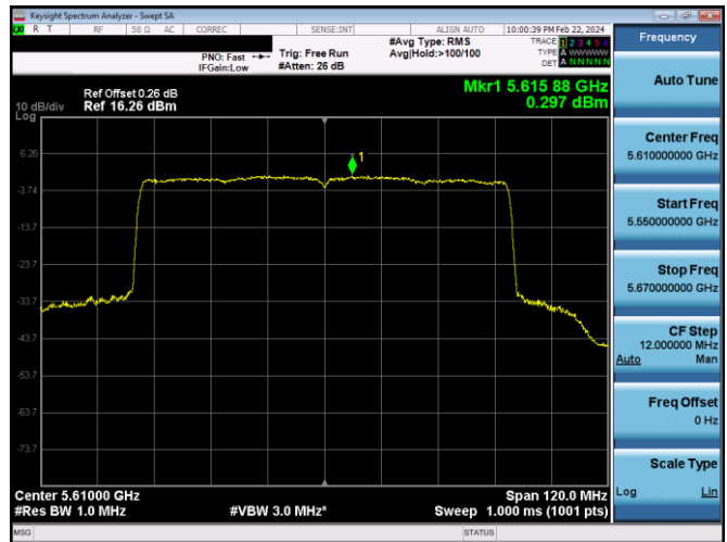
Plot 7-822. PSD CDD DIVERSITY Antenna WF7 (80MHz BW 802.11ax(SU) – Ch. 122, MCS4)
