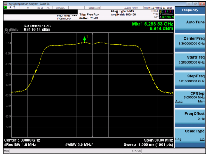
Plot 7-593. PSD CDD PRIMARY Antenna WF5b (20MHz BW 802.11n - Ch. 60, MCS10)
