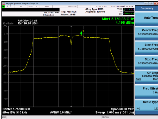
Plot 7-537. PSD Antenna WF7 (40MHz BW 802.11n – Ch. 151, MCS2)
