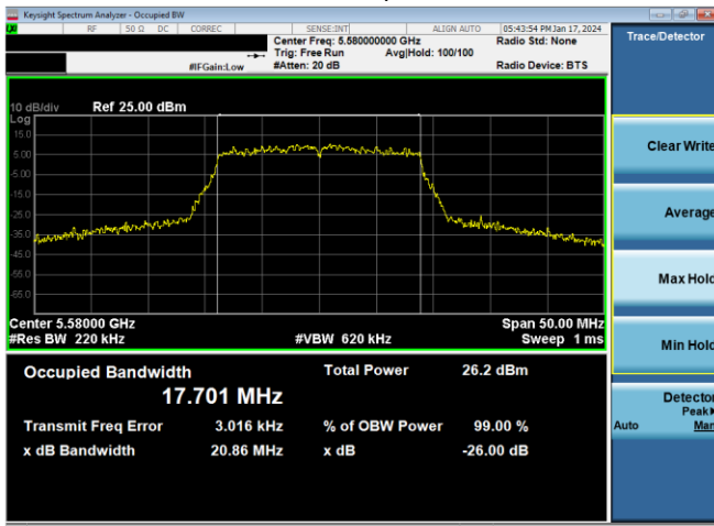
Plot 7-37. 26dB BW & 99% OBW Antenna WF5b (20MHz BW 802.11n – Ch. 116, MCS4)
