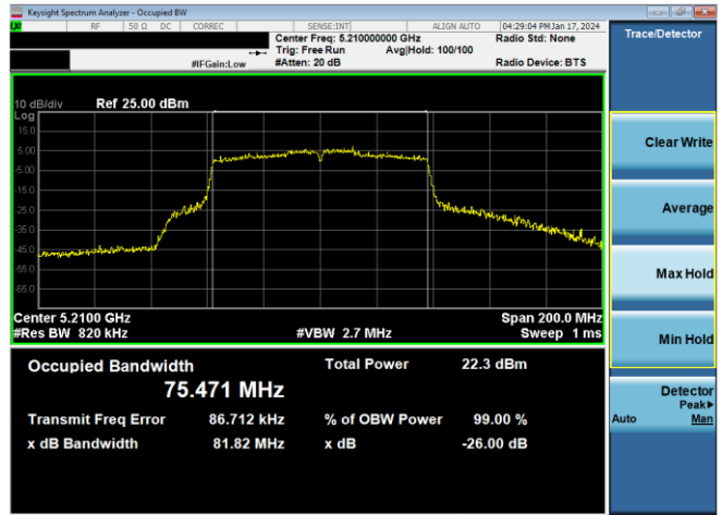
Plot 7-5. 26dB BW & 99% OBW Antenna WF5b (80MHz BW 802.11ac – Ch. 42, MCS2)
