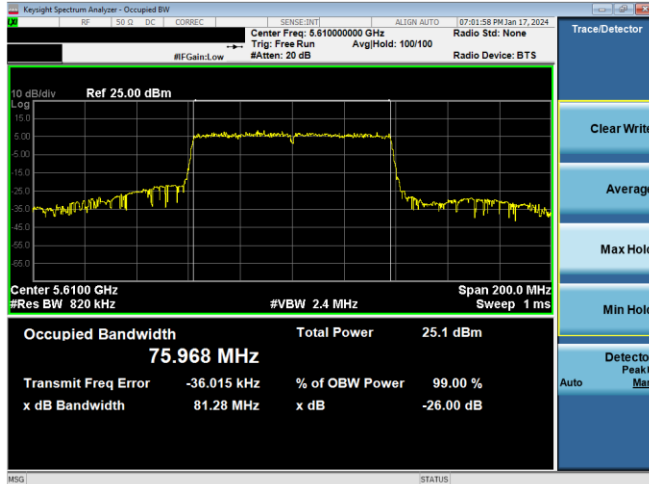
Plot 7-63. 26dB BW & 99% OBW Antenna WF5b (80MHz BW 802.11ac – Ch. 122, MCS9)
