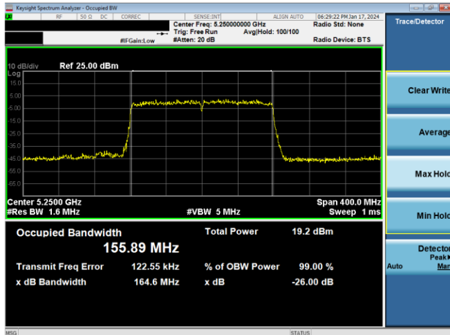
Plot 7-52. 26dB BW & 99% OBW Antenna WF5b (160MHz BW 802.11ac – Ch. 50, MCS11)
