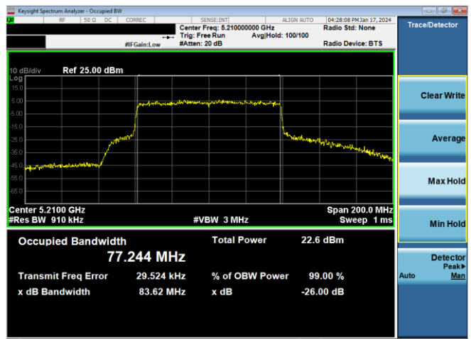
Plot 7-6. 26dB BW & 99% OBW Antenna WF5b (80MHz BW 802.11ax(SU) – Ch. 42, MCS2)
