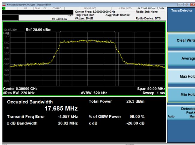
Plot 7-9. 26dB BW & 99% OBW Antenna WF5b (20MHz BW 802.11n – Ch. 60, MCS2)
