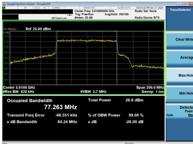
Plot 7-20. 26dB BW & 99% OBW Antenna WF5b (80MHz BW 802.11ax(SU) – Ch. 122, MCS2)
