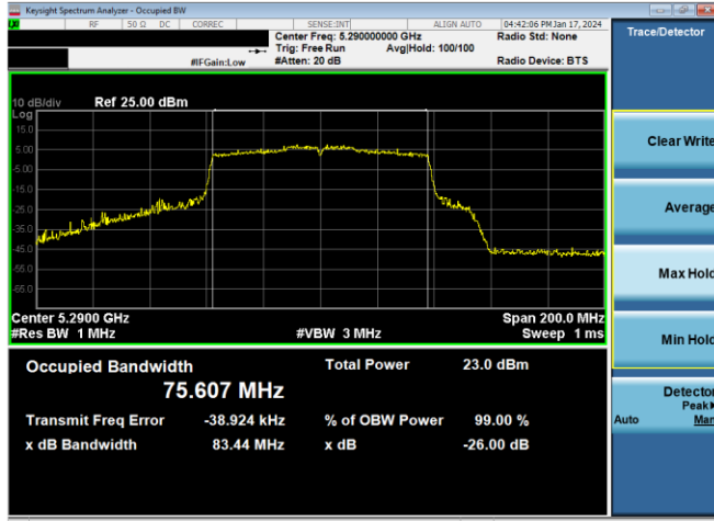
Plot 7-13. 26dB BW & 99% OBW Antenna WF5b (80MHz BW 802.11ac – Ch. 58, MCS2)
