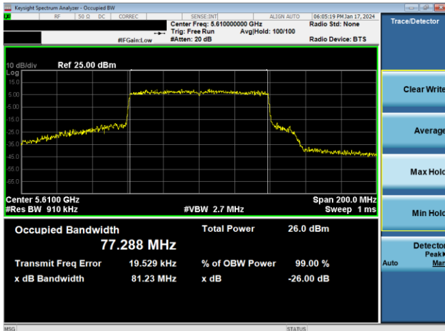
Plot 7-42. 26dB BW & 99% OBW Antenna WF5b (80MHz BW 802.11ax(SU) – Ch. 122, MCS4)
