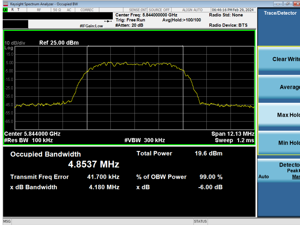
Plot 7-30. 6dB BW & 99% OBW Antenna WF8 (HDR8, ePA, 5844MHz)
