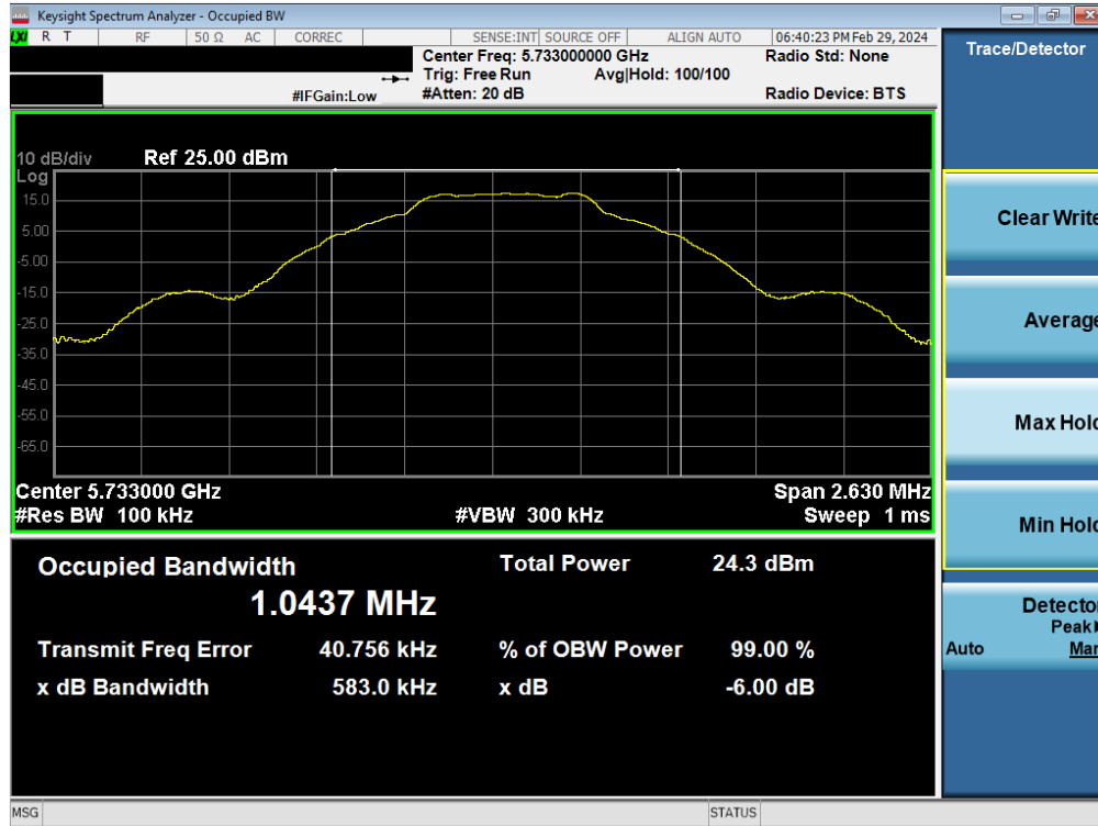
Plot 7-13. 6dB BW & 99% OBW Antenna WF8 (BDR GFSK, 5733MHz)
