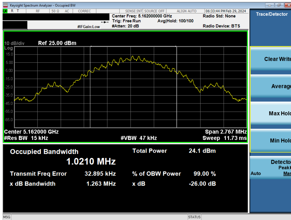
Plot 7-4. 26dB BW & 99% OBW Antenna WF8 (BDR GFSK, ePA– 5162MHz)
