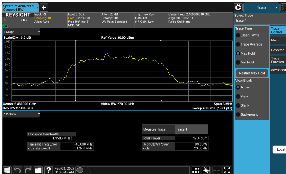
Plot 7-6. 20dB BW and 99% OBW Plot (Bluetooth, 8DPSK – Ch. 78)
