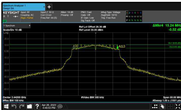
Figure 55 - 802.11g Minimum 6 dB EBW
