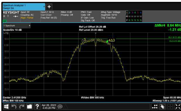
Figure 53 - 802.11b Minimum 6 dB EBW
