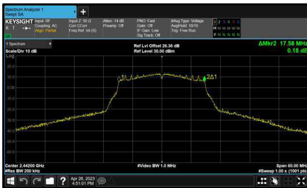
Figure 65 - 802.11n HT20 Minimum 99% OBW
