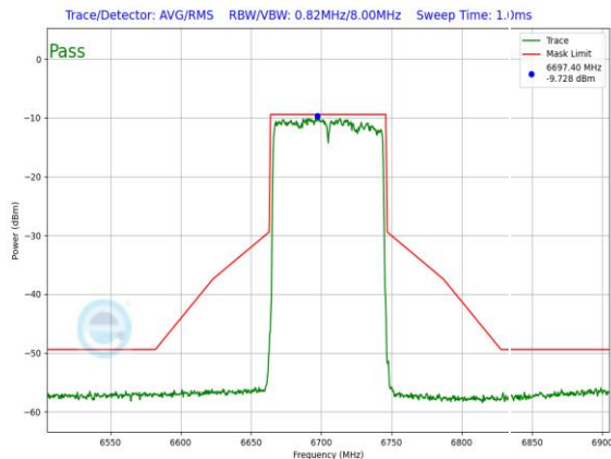
Plot 7-1495. LPI In-Band Emission Plot SDM Diversity Antenna 3c (80MHz) 802.11ax RU996 (UNII Band 7) – Ch. 151
