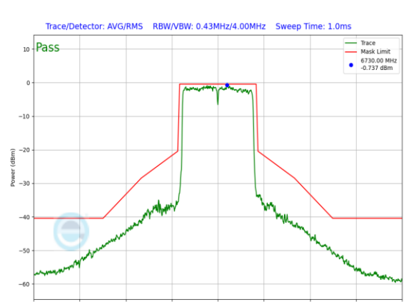
Plot 7-952. SP In-Band Emission Plot Antenna 1b (40MHz 802.11ax RU484 (UNII Band 7) – Ch. 155)
